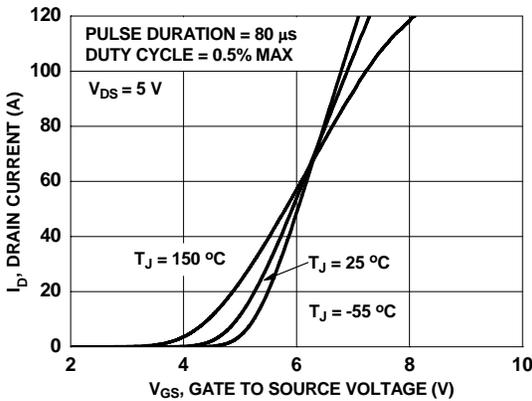
Figure 5. Transfer Characteristics
