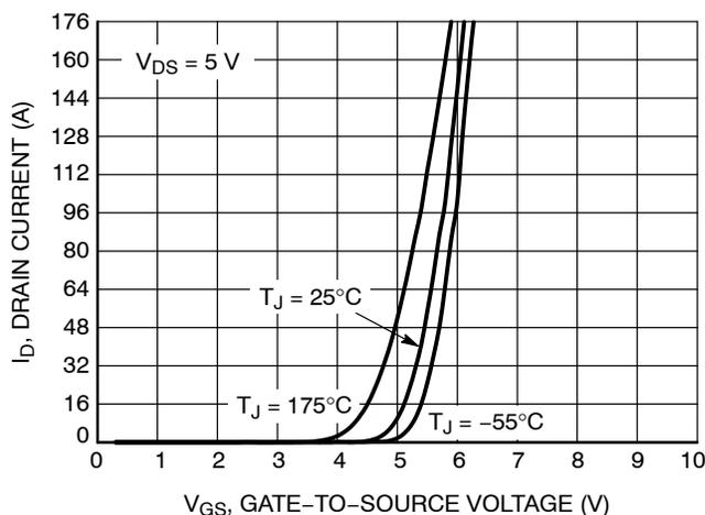
Figure 2. Transfer Characteristics
