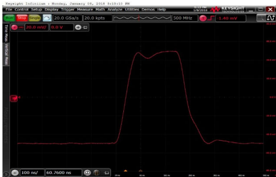
Voltage: 20 mV/div, Time: 100 ns/div V_S = \pm 15\text{ V} , R_L = 2\text{ k}\Omega , C_L = 100\text{ pF} , G = 1
