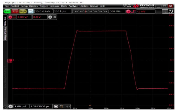
Voltage: 2 V/div, Time: 1 \mu s/div V_S = \pm 15\text{ V} , R_L = 2\text{ k}\Omega , C_L = 100\text{ pF} , G = 1
