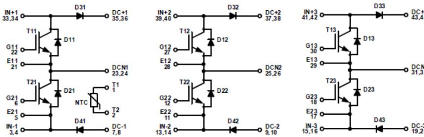
Figure 2: Schematic diagram of [NXH600B100H4Q2F2](#) 3 Channel Symmetric Boost module design.
