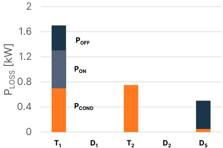
Figure 3: Power loss distribution of I-NPC when PF=1
