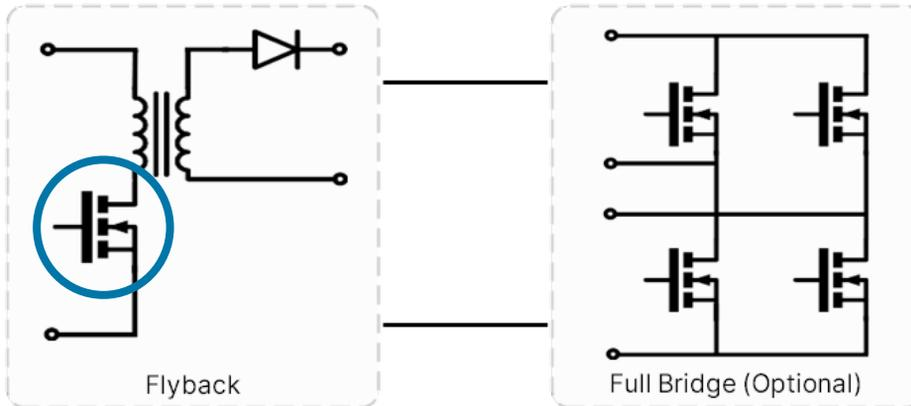
Figure 1: Simplified Power Conversion Stages of a Micro Inverter
