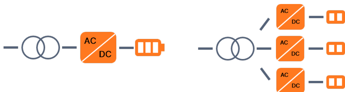
Figure 1: Centralized and Distributed BESS Solution
