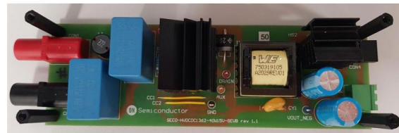
Figure 5: Example Schematic based on NCP1362 flyback controller (above) Evaluation Board with NCP1362 (below)
