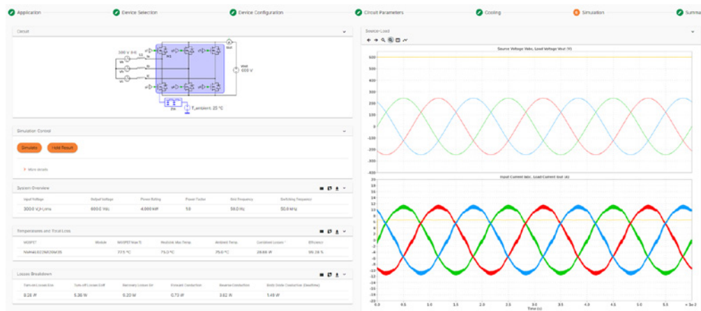
Figure 4. Elite Power Simulator: Simulation Results and Waveforms
