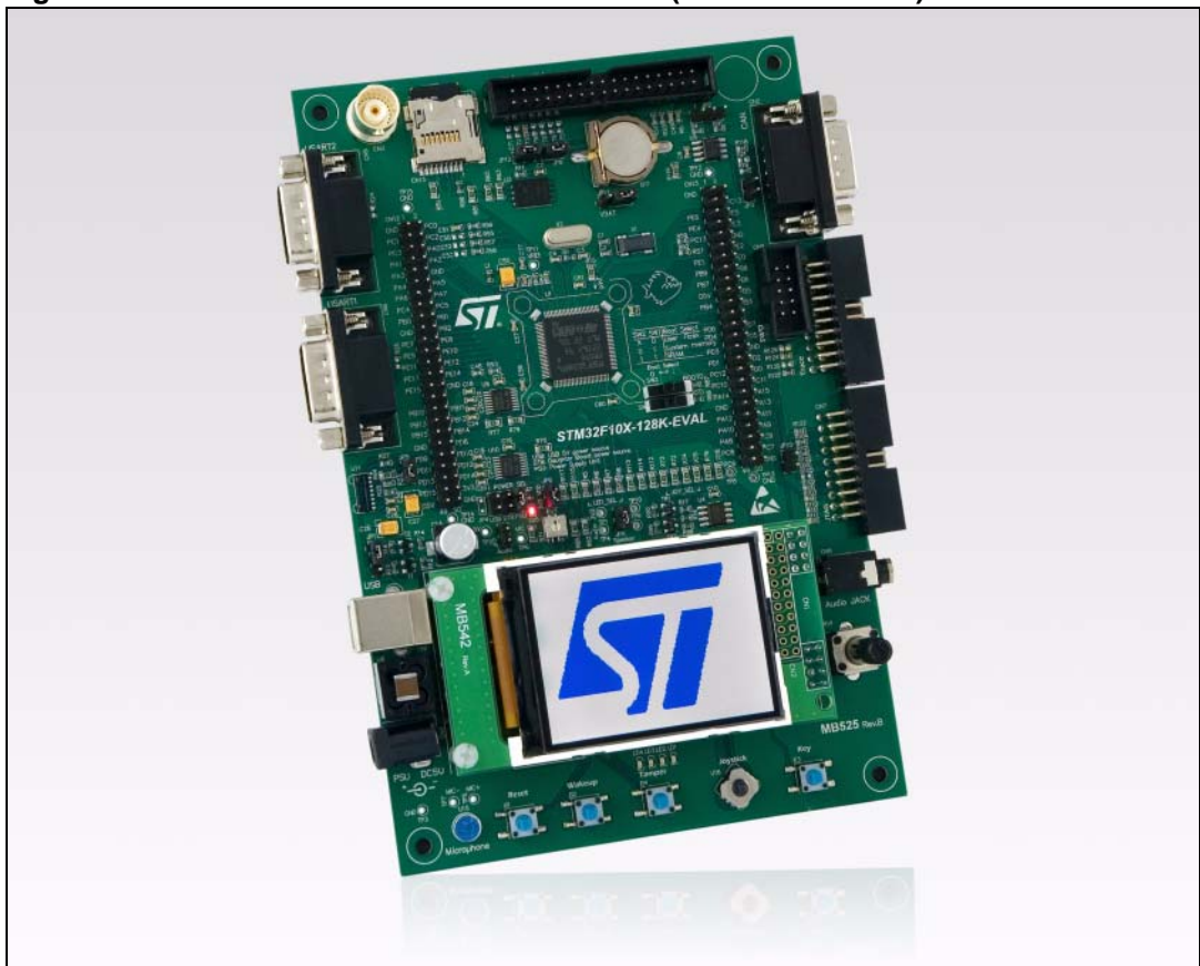
Figure 1. STM32F10X 128K evaluation board (STM3210B-EVAL)
